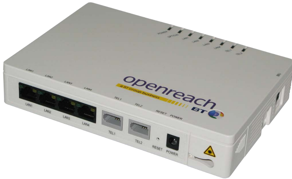
Figure 3 – Type 2 ONT showing ports and LEDs
