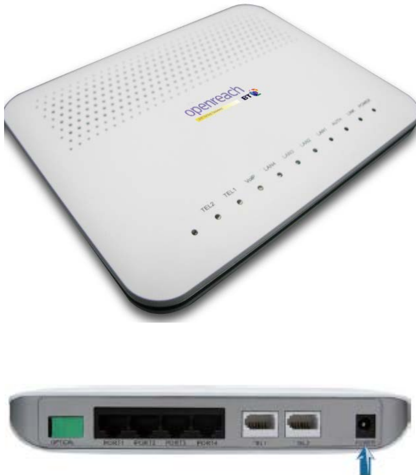
Figure 3 – Type 1 ONT showing ports and LEDs
