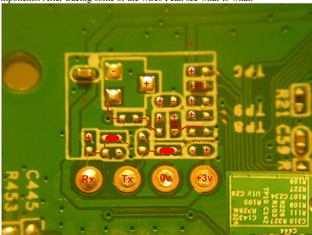
I bridged the thicker red lines (R327 & R328) and used the normal parameters:
